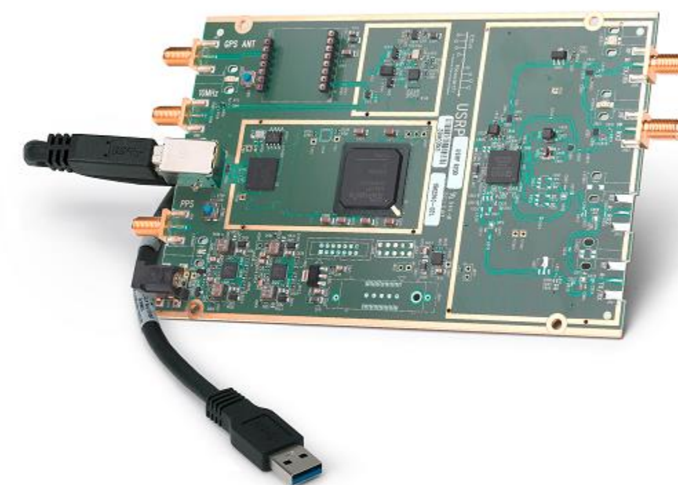
Figure 2 – The USRP B200 radio used to generate and send the RF signal to the rest of our device.
