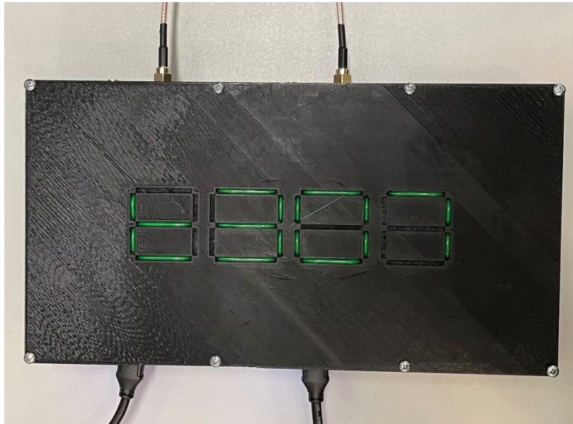
Figure 1: Prototype I/O (two input SMA cables on the top, and two output USB 2.0 cables on the bottom).
