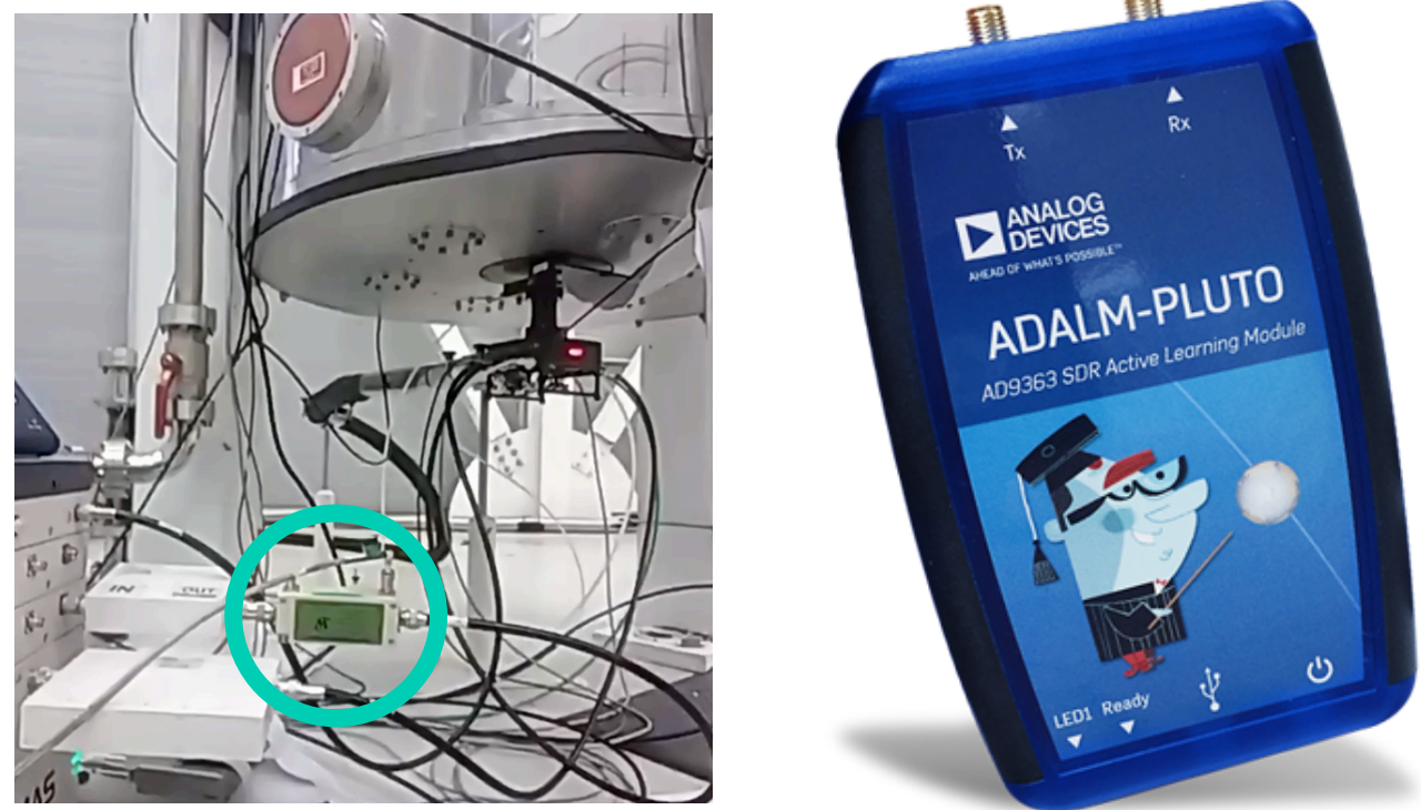
Figure 1. NMR probe & Bidirectional Coupler (left); Adalm-Pluto SDR (right)
