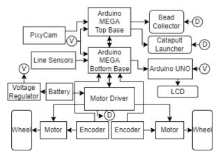
The diagram above is an overview of the connections between the modules on the robot. The robot consists of two tiers: the top base and the bottom base. Each tier has its own general purpose, with the bottom base serving mainly as a navigational and power module and the top base serving as a functions module, with the image recognition, catapult, and the arm.
