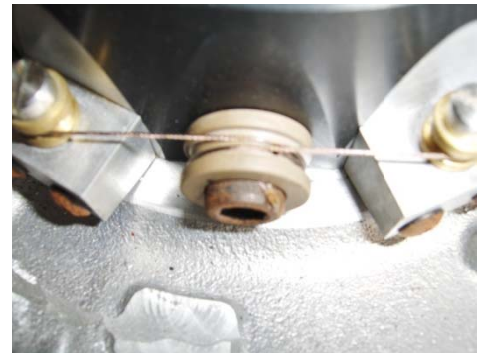
Figure 4 – Idler Block and IGV Pulley Set Up
