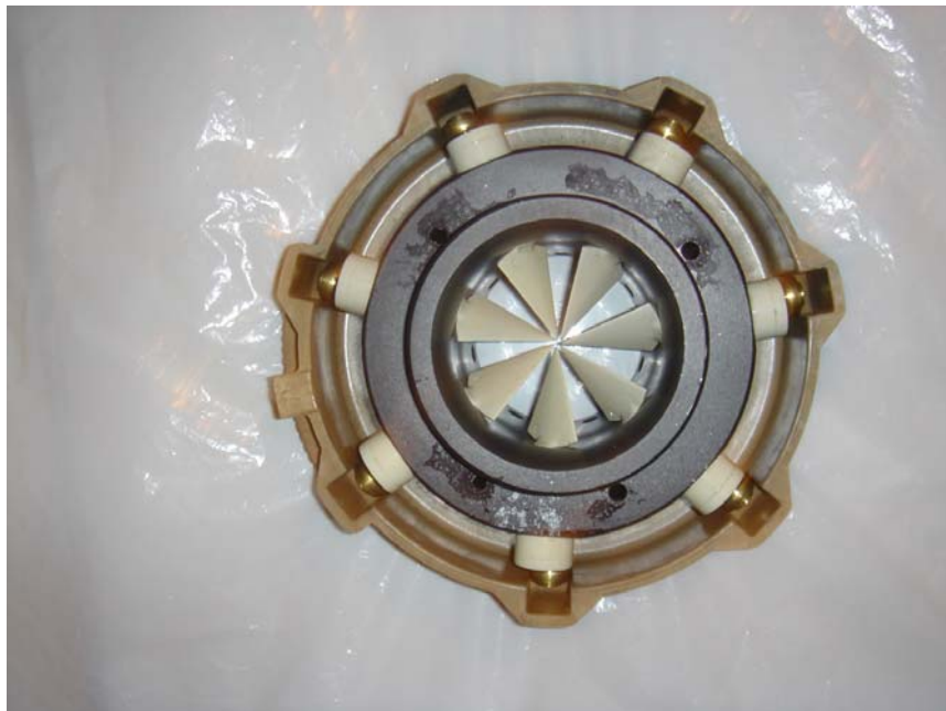
Figure 1.1 – The Housing with the throat, IGV and cam arms attached. The Black part is the throat, the cam rollers can be seen in the slots of the housing, and the IGV are the triangular shaped pieces in the middle.
