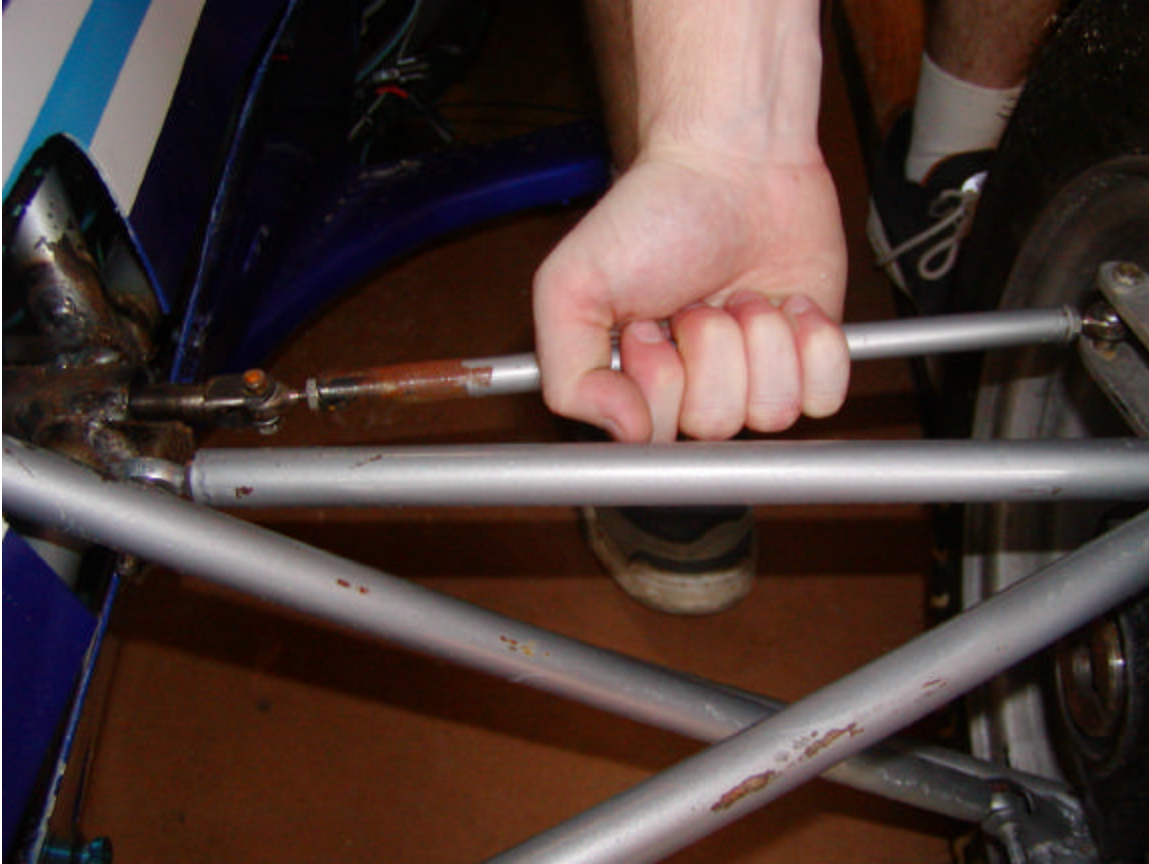
Figure 5: Front Toe Adjustment
