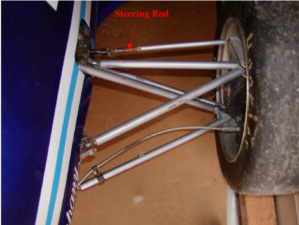
Figure 4: Front Suspension with Steering Rod Shown
