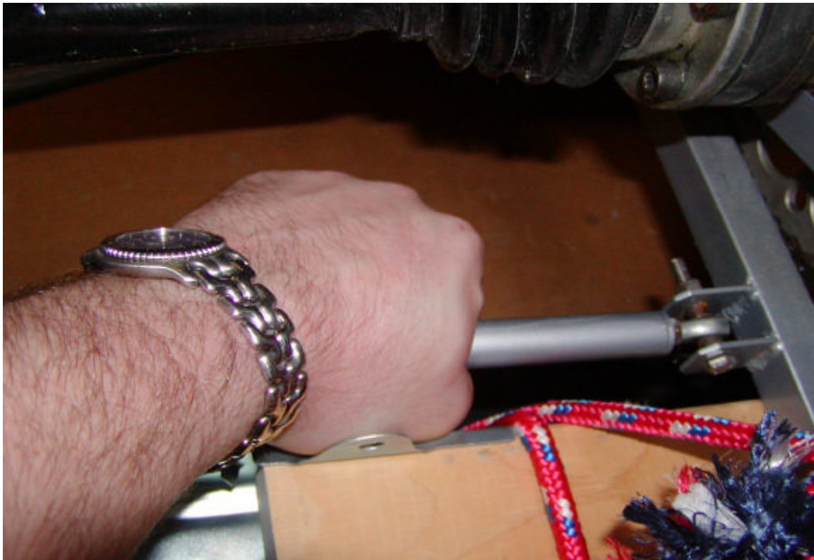
Figure 7: Rear Toe Adjustment
