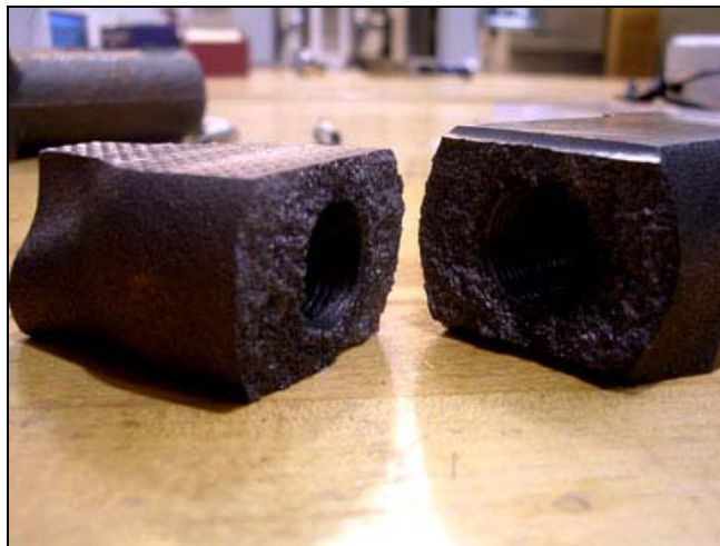
Figure 11: Main bearing cap test, engine block failure.
