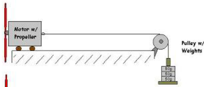
Figure 14- Testing rig for thrust using a pulley and weights
