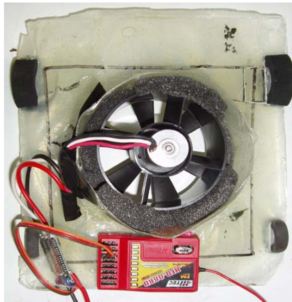
Figure 16- Mockup of design to use for vertical wall testing
