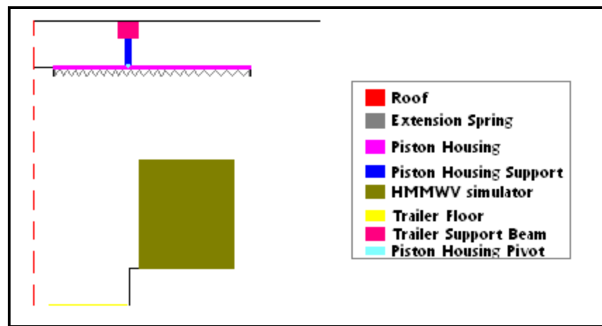
Figure E-7: Schematic of Pneumatic Cylinder Setup
