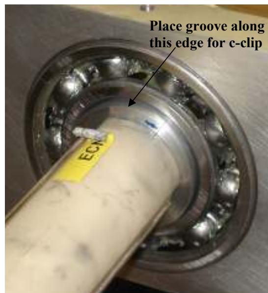
Figure 12-1 – View of slit collar with possible position for c-clip retaining ring
