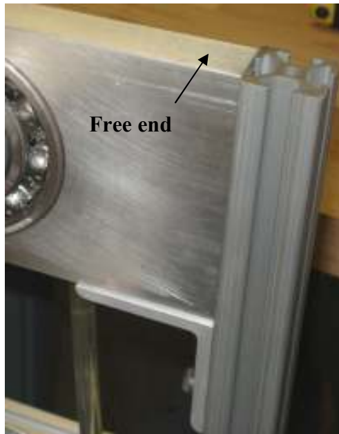
Figure 12-2 – Picture of bearing-plate showing its L-bracket support (4-bolts, two on each side, not fully shown).
