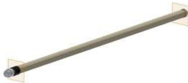
Figure 5-4 – Shaft shown with planes where radial displacement may be observed in two-plane balance detection.
