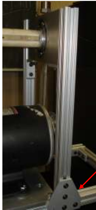
Figure 12-3 – Picture of vertical arm used on the bearing-plate side of machine.
