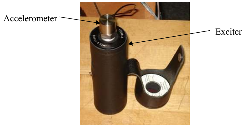
Figure 9-5 – Picture of exciter with accelerometer installed.
