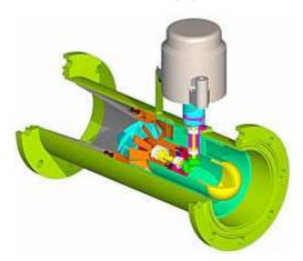
**Axial-tubular micro hydropower unit.** It was designed and manufactured in order to fit an isolated micro hydropower station. It is intended for some stations where the discharge  $Q_C$  is 112...130 l/s, and the head H c is within 3...3.5 m. The resulted power is of 4 kV. It is designed in a solid construction with no pollutant conditions, its housing being performed
