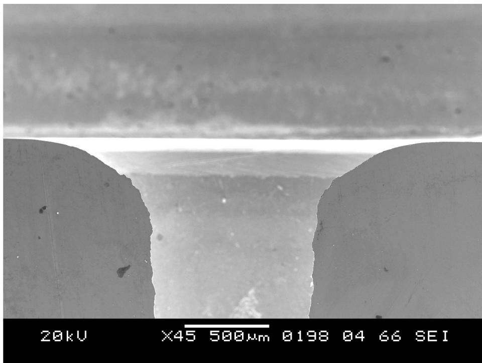
SEM vertical cross section picture of polished plunger at 45x
