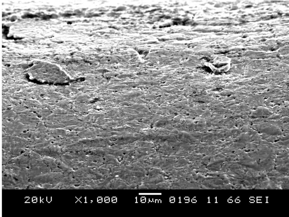
SEM overhead picture of unpolished plunger at 1000x
