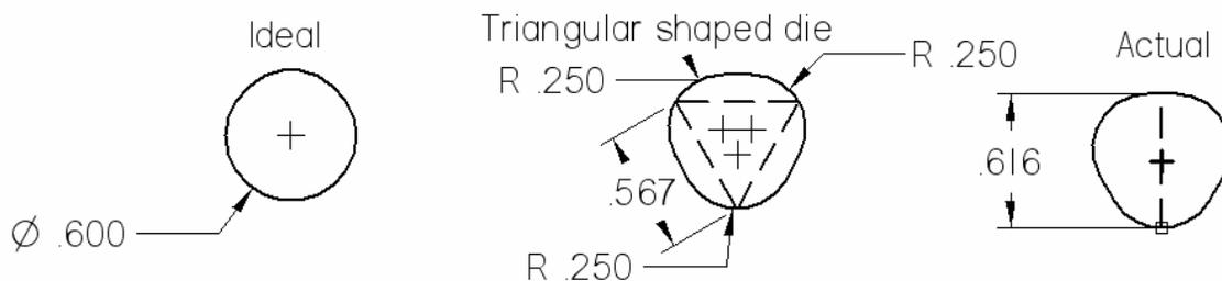
*These dimensions are not accurate to the design specifications and are exaggerated to demonstrate the concept.*
