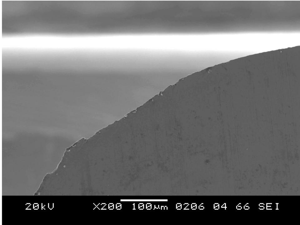
SEM vertical cross section picture of polished plunger at 200x
