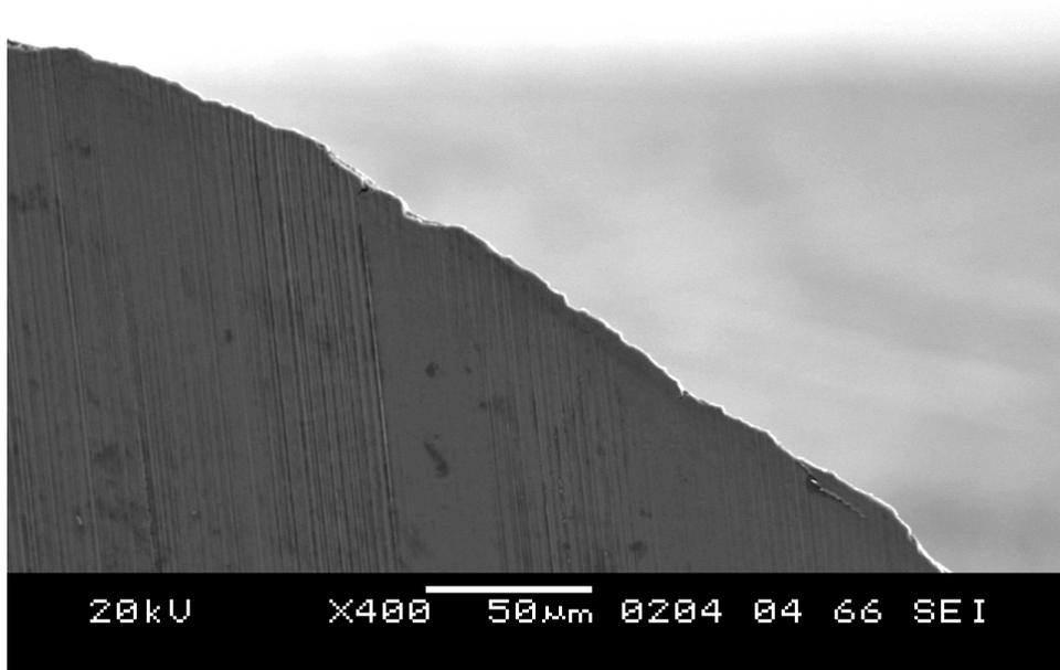
SEM vertical cross section picture of unpolished plunger at 40x
