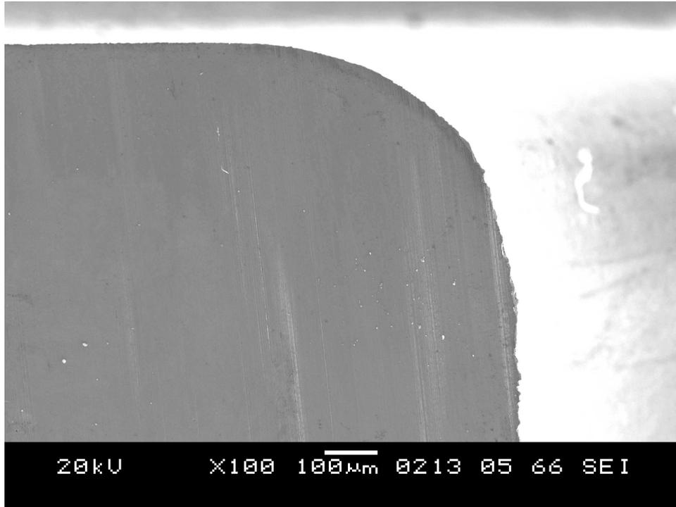
SEM vertical cross section picture of unpolished plunger at 100x
