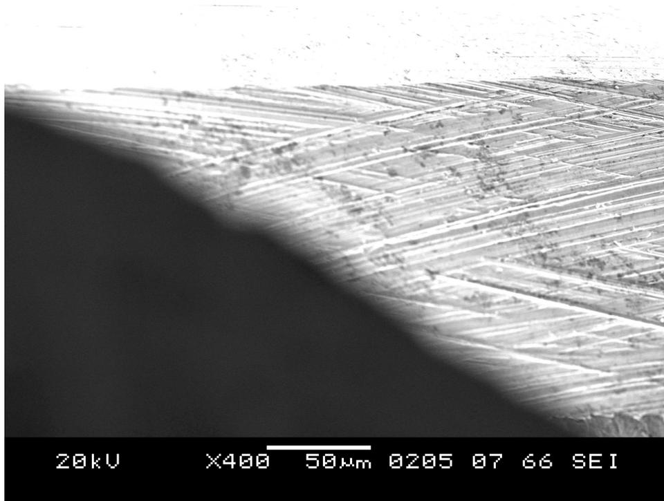
SEM vertical cross section picture of polished plunger at 400x
