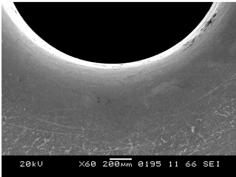
SEM overhead picture of unpolished plunger at 60x
