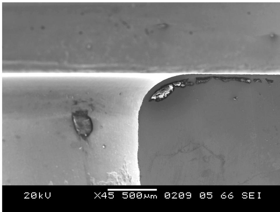
SEM vertical cross section picture of unpolished plunger at 45x
