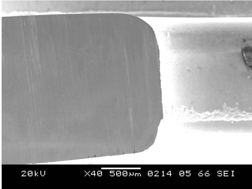
SEM vertical cross section picture of unpolished plunger at 40x
