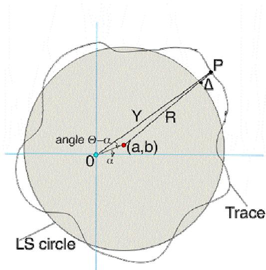
Improvements to the quality here will be the addition of a measurement system that quantifies the roundness of the hole to see that they are within the specified limit. Calculating the roundness can be done by tracing the circular surface, in this case the valve seat. This can be done by a mechanical stylus or an optical laser. Lasers provide higher speed, precision, and accuracy and could simultaneously
