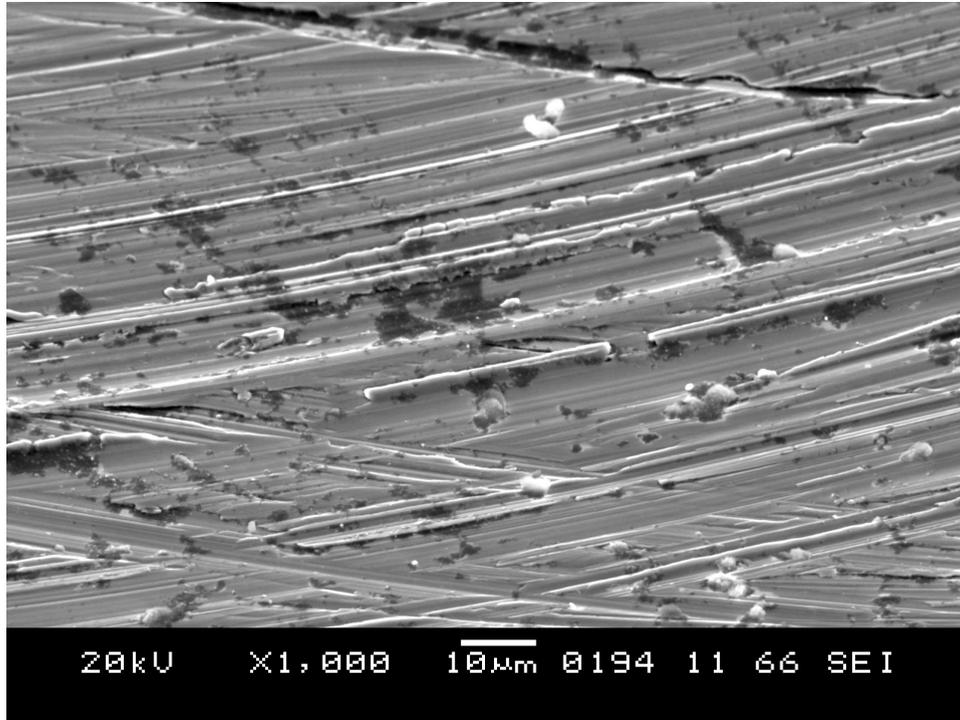
SEM overhead picture of Polished Plunger at 1000x
