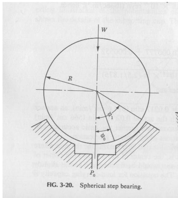
FIG. 3-20. Spherical step bearing.
