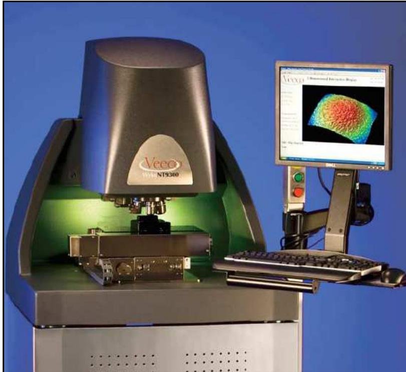
Through extensive research, the Wyco NT-9300 (see appendix \_\_\_ for technical specifications) was determined to be the most suited machine for the job required at GT Technologies. This model is produced by Veeco, one of the world leaders in 3D metrology. Their expertise includes nano-scale imaging, LCD technology, and automated profiler systems. The reasoning behind this choice was simply the advantages that optical profilers have in an assembly line.
