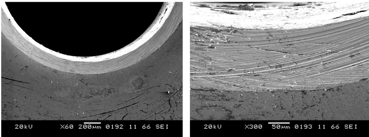
A side effect of polishing the plunger seat is that the radius of the check ball is imposed onto the seat, which provides more surface area for the check ball to sit. Once, the manufacturer heat treated the plungers. This was a necessary step to remove carbide scale that would adversely affect product performance.
