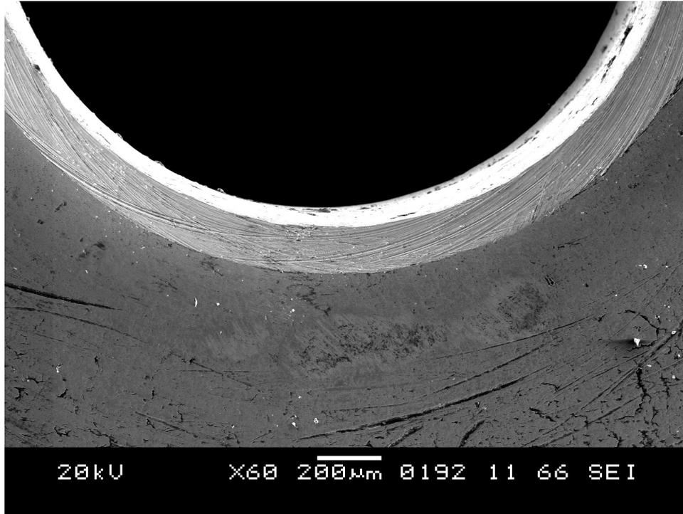
Scanning Electron Microscope (SEM) overhead pictures of Polished Plunger at 60x
