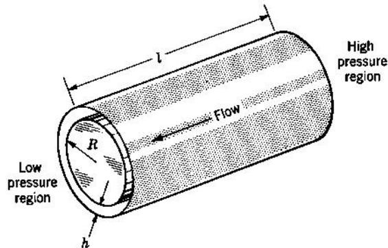
FIG. 2-18. Capillary seal.
