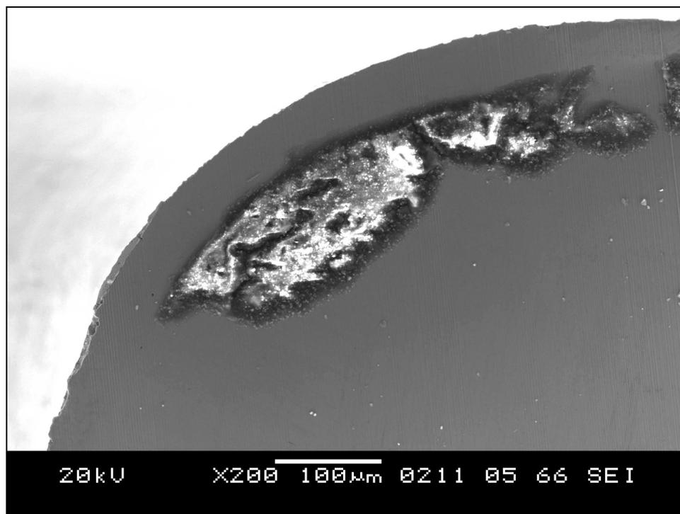
SEM vertical cross section picture of unpolished plunger at 200x
