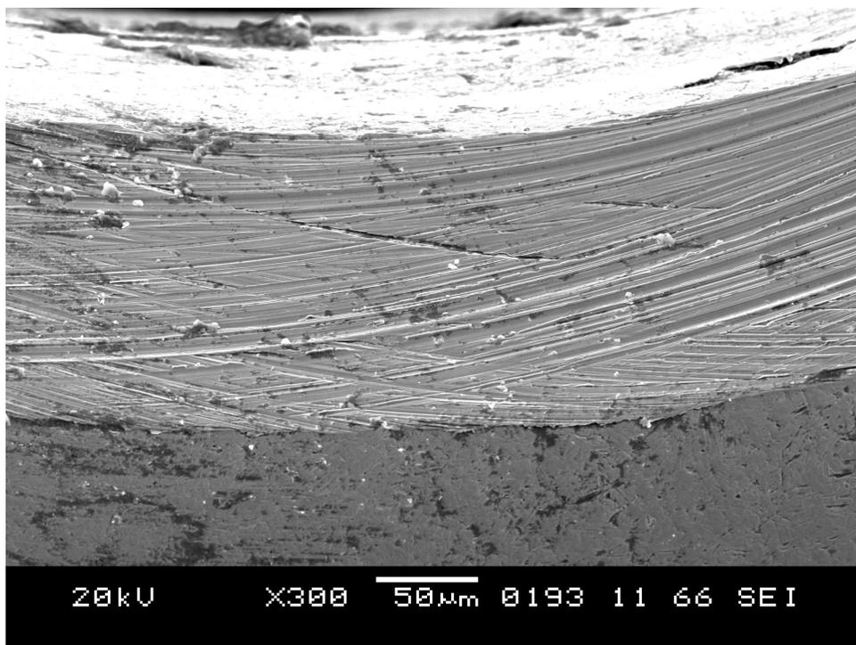
SEM overhead picture of Polished Plunger at 300x
