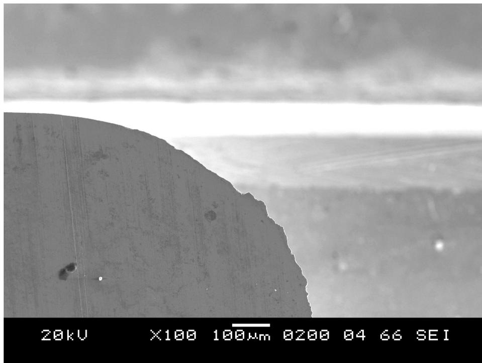
SEM vertical cross section picture of polished plunger at 100x
