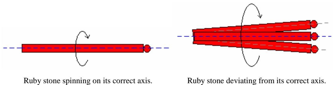
The wobbling problem stems from lack of support necessary support in the ruby stone holder. If the stone's deviation is drastic enough, it can ultimately damage the plunger's oil-tight seal; rendering the plunger un-usable. And of course, the more parts that fail quality control testing, the more money GT is wasting.
