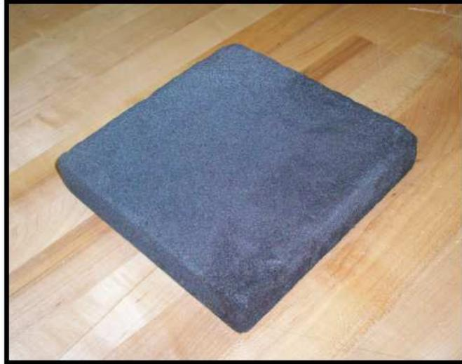
*Figure 2.2.b.1: Carbon Foam Conduction Element*
