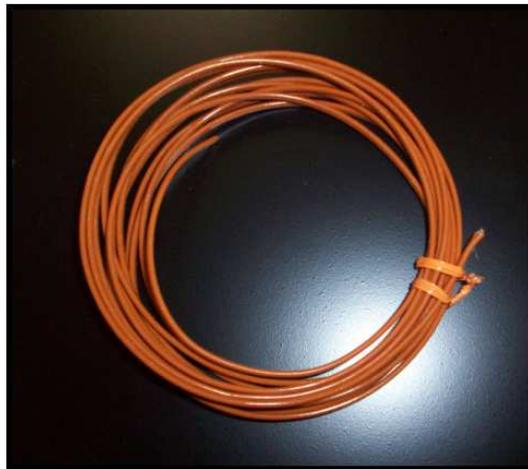
*Figure 6.2.b.2: Thermocouple Wire Used to Manufacture Thermocouples*
