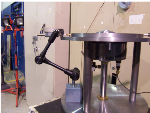
Figure 22: Profile view of the magnet dial gauge attached to the test rig for concentricity measurements.
