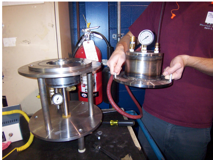
Figure 20: Picture showing the high pressure vessel separated from the rest of the rig
