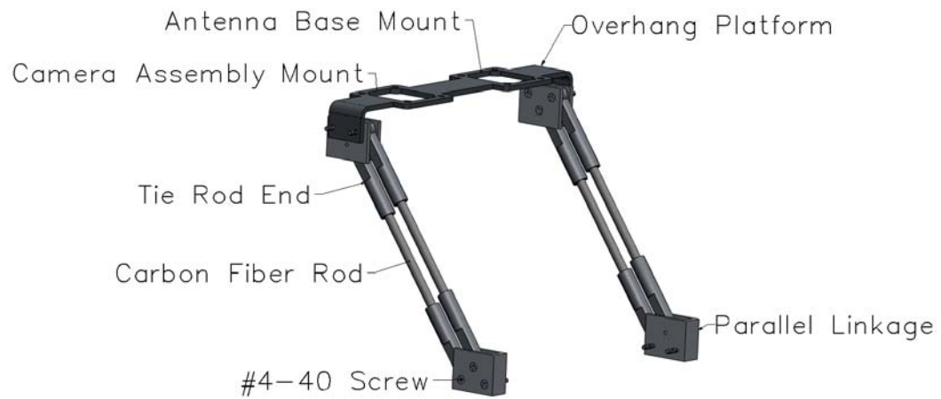
Figure 15: Detailed Design of Swinging Platform
