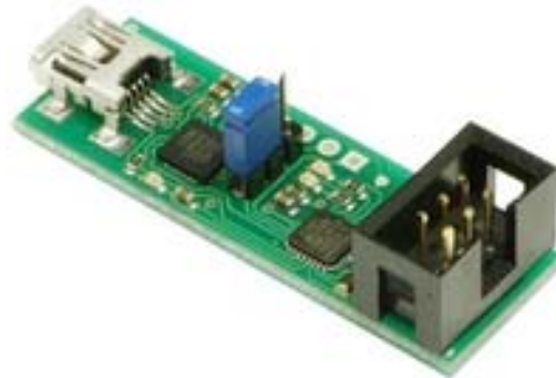
Figure 24: Orangutan USB Programmer
