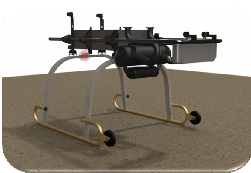
Figure 2: Rendered Solid Model of RMAX Skids representing Yamaha RMAX
