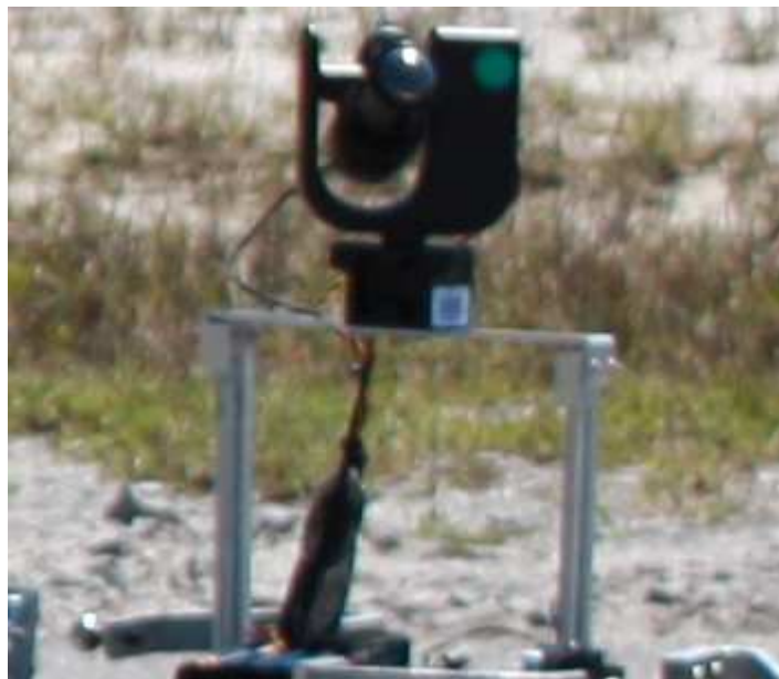
Figure 44: Aluminum arms for swinging platform
