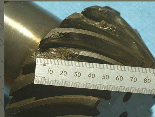
Fig. 1 – Worn Bevel Gear Teeth
