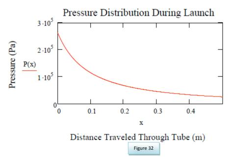
Once the pressure was determined, the instantaneous Gs the UAV and carriage experience during the launch process were calculated. This is for an exit velocity of 19.812 m/s, a forty-five degree launch angle, and an initial pressure of .2461 MPa. The instantaneous acceleration ranged from 150.028 down to only 17.099 Gs during the launch. The instantaneous acceleration in which the UAV and carriage will experience has been simulated and the data can be seen below Figure 33.
