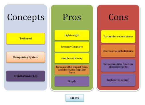
Due to weight restrictions, the dampening system and the rigid lip cylinder were ruled out. The cable was also a more simple design and less costly than the other two designs. The rigid cylinder lip has the potential to inflict damage on both the carriage and itself. Once the team decided to use the cable, one needed to be found that would satisfy all of the requirements.
