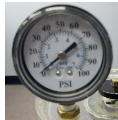
Figure 3 - Pressure Gauge Mounted to Backing
