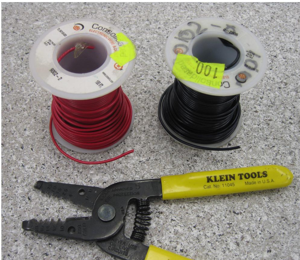
Figure 3-4: Red and black 16 awg wire and wire stripping tool
