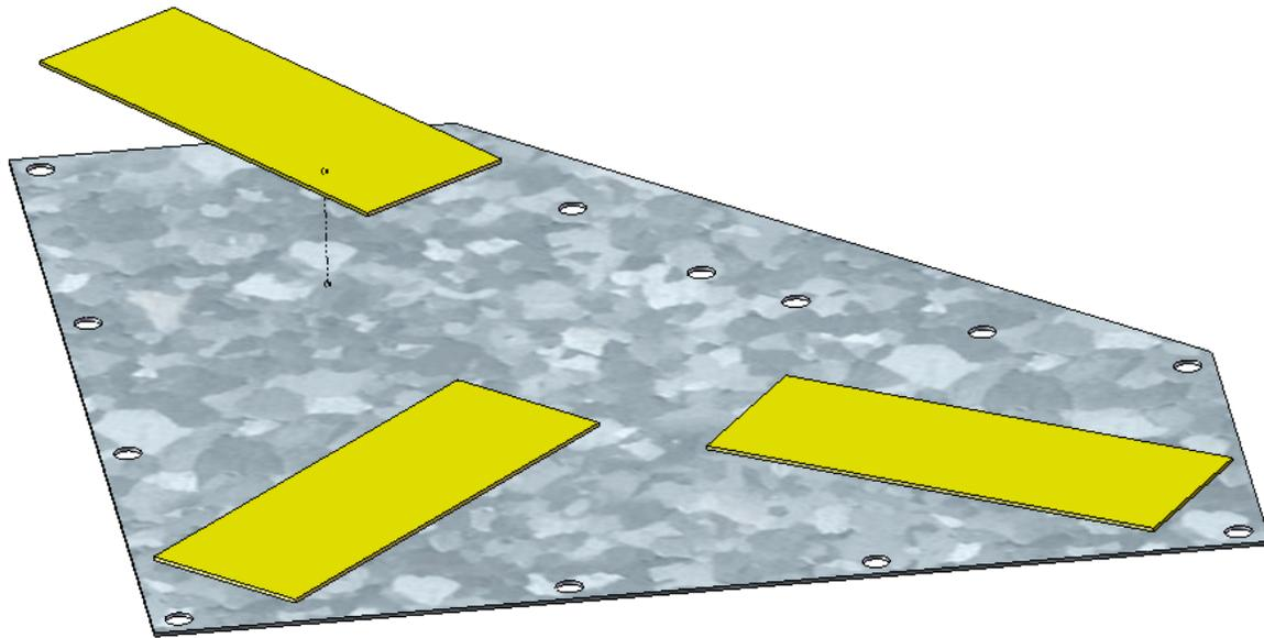
Figure 3-2: MFC orientation on scale model cover
