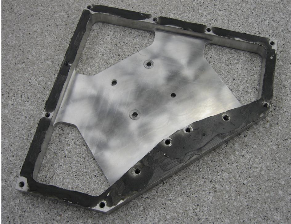
Figure 3-7: Scale model housing with black RTV sealant
