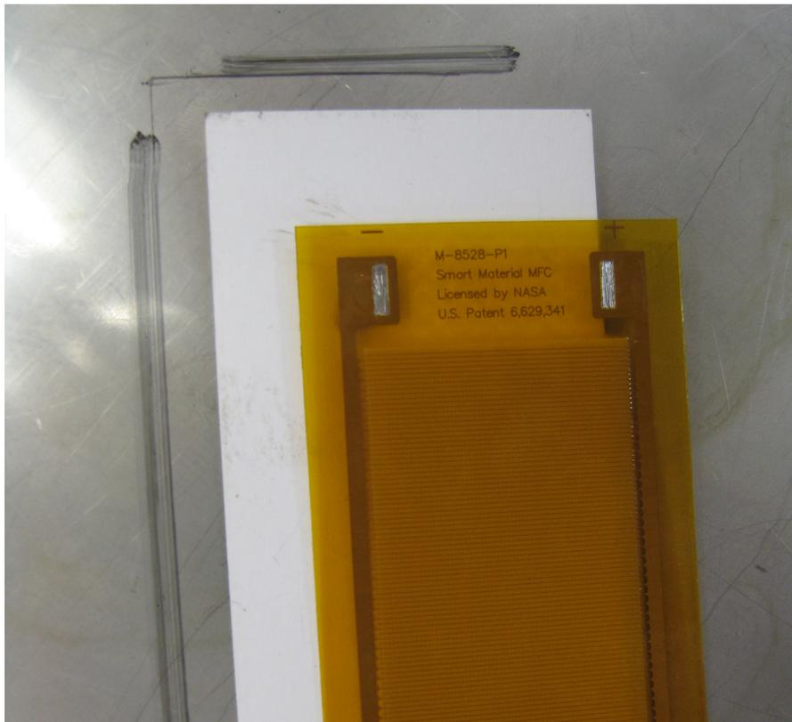
Figure 3-3: MFC, MFC cutout, and stencil marking
