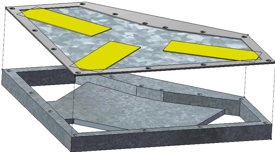
Figure 3-8: Scale modeling cover positioned above scale model housing
