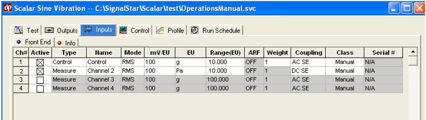
Figure 4-10: Screenshot of the Inputs portion of the Test Setup menu
