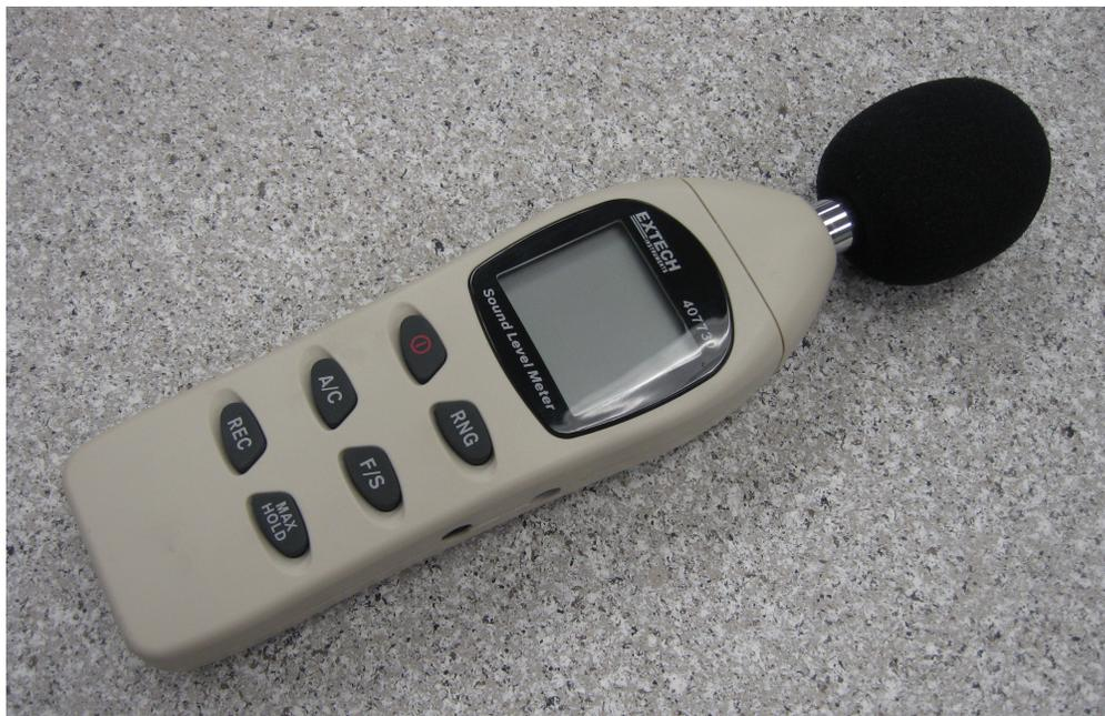
Figure 4-2: Extech sound level meter
