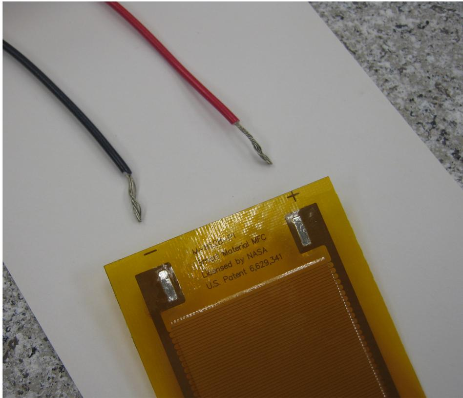
Figure 3-5: MFC positive and negative contact patches
