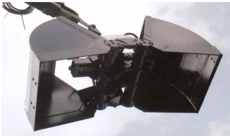
Figure 2.2b. Clamshell attachment for backhoes [30].
