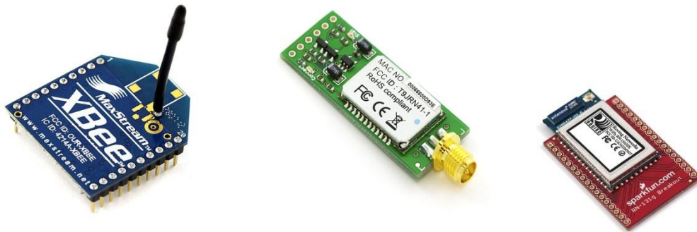
Figure 2.6b. Modules for interfacing a microcontroller with Zigbee, Bluetooth and Wi-Fi respectively [20, 21, 22].
