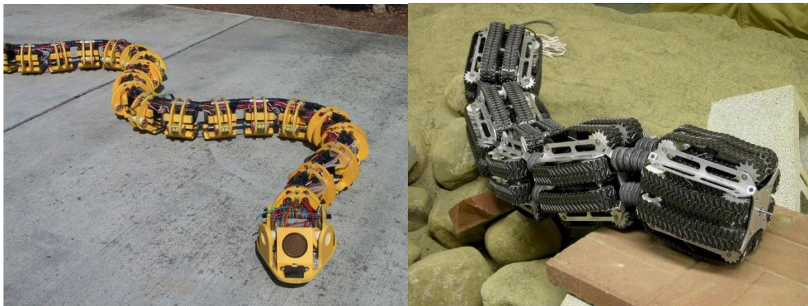
Figure 2.4d. (left) Example of worm-like locomotion in SnakeBot [8]. (right) Another example of possible worm locomotion using multiple tiers of tracks on the OmniTread Serpentine Robot [7].
