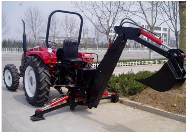
Figure 2.2g. A standard backhoe mounted to a tractor [25].
