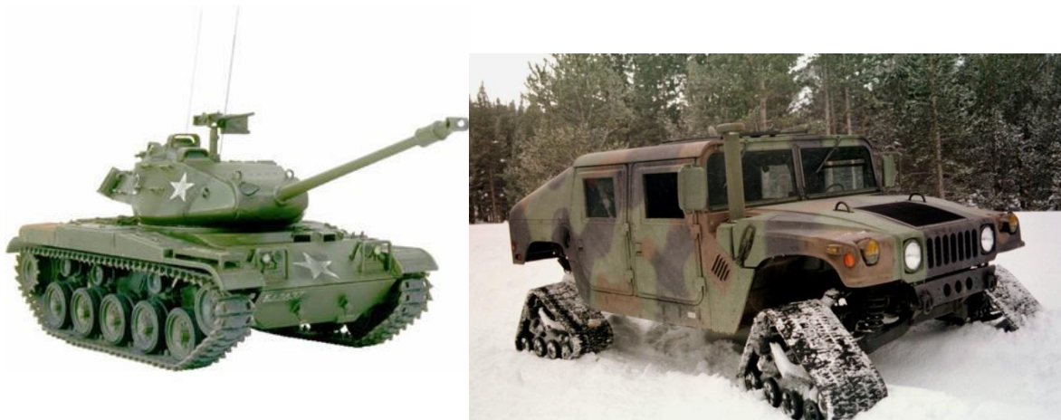
Figure 2.4b. (left) Tracks have been implemented on military vehicles such as tanks for almost a century [4]. (right) Tracks have been adapted to a variety of vehicles and uses, as shown being utilized by a humvee for off-road, winter conditions [3].
