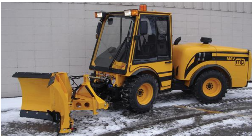
Figure 2.2f. An adjustable v-plow in inward-v position [24].
