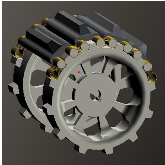
Figure 4.2b. Example of treads wrapping around sprocket of locomotion system.
