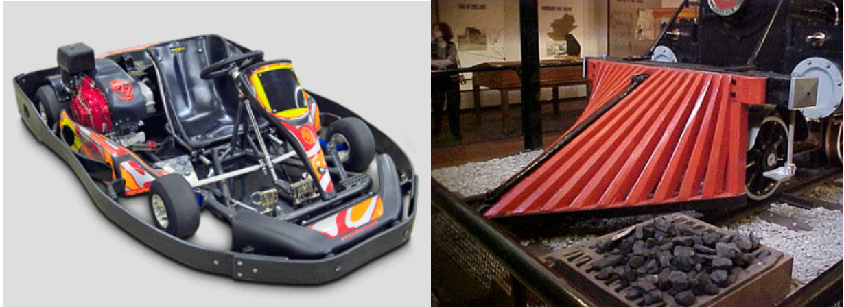
Figure 2.3a. (left) Wraparound bumper on go-kart. (right) Pilot (cowcatcher) on locomotive [33,34].
