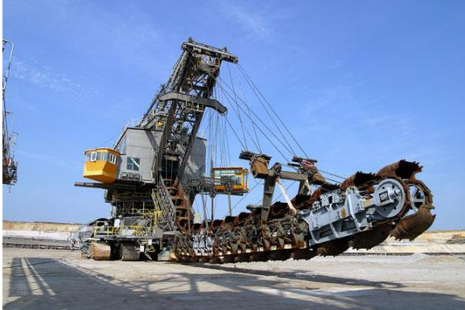
Figure 2.2a. Commercial bucket chain excavator [29].
