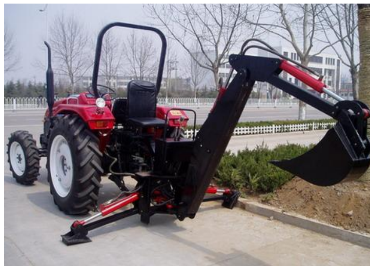
Figure 10. A standard backhoe mounted to a tractor [25].
