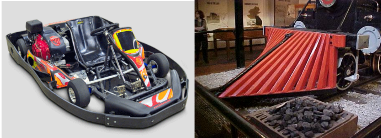
Figure 13. (left) Wraparound bumper on go-kart. (right) Pilot (cowcatcher) on locomotive [33,34].
