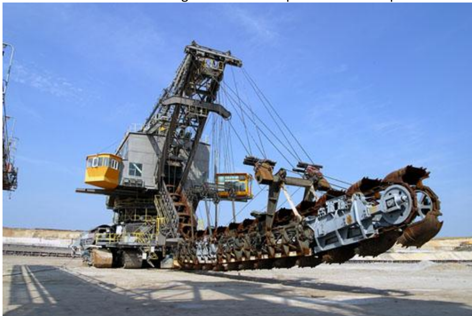
Figure 4. Commercial bucket chain excavator [29].
