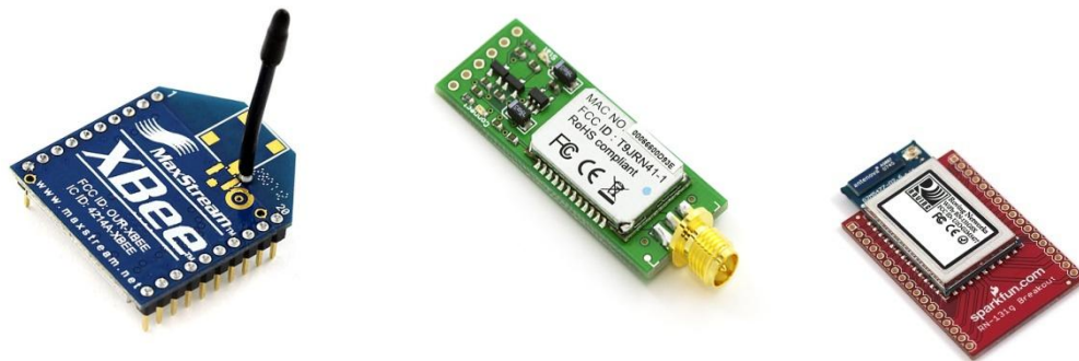
Figure 21. Modules for interfacing a microcontroller with Zigbee, Bluetooth and Wi-Fi respectively [20, 21, 22].
