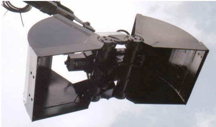
Figure 5. Clamshell attachment for backhoes [30].
