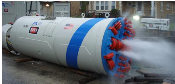
Figure 7. Microtunneling Boring Machine [32].
