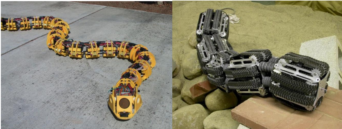
Figure 18. (left) Example of worm-like locomotion in SnakeBot [8]. (right) Another example of possible worm locomotion using multiple tiers of tracks on the OmniTread Serpentine Robot [7].
