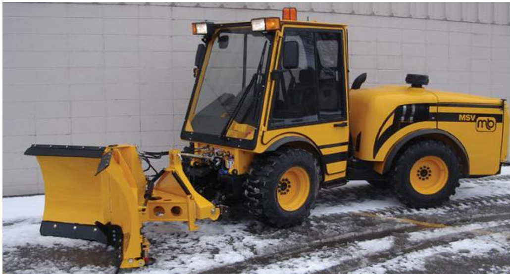
Figure 9. An adjustable v-plow in inward-v position [24].
