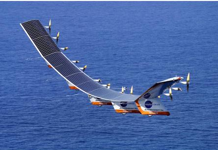
NASA Dryden Flight Research Center Photo Collection http://www.dfrc.nasa.gov/gallery/photo/index.html NASA Photo: ED01-0209-3 Date: July 14, 2001 Photo by: Nick Galante/PMRF The Helios Prototype flying wing is shown over the Pacific Ocean during its first test flight on solar power from the U.S. Navy's Pacific Missile Range Facility in Hawaii.
