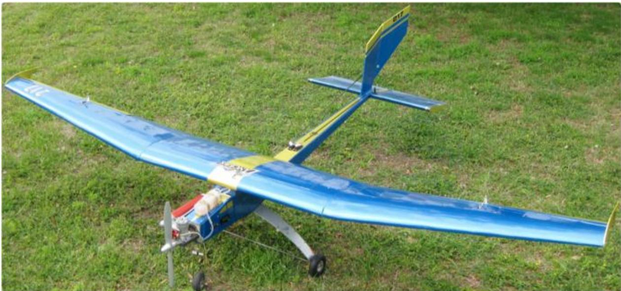
**Figure 3.1: Example of a conventional design with a tricycle main gear configuration**
