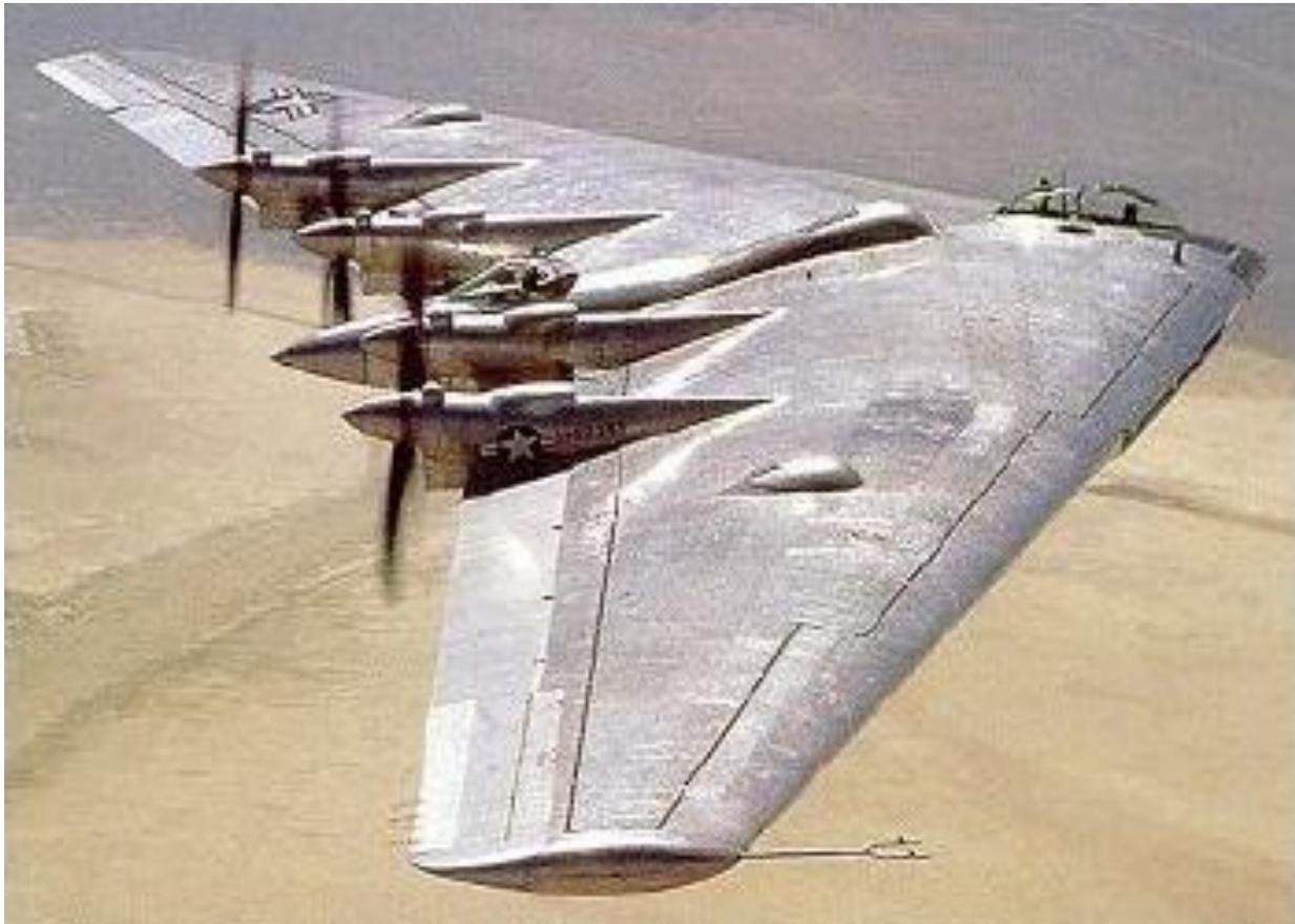
Figure 3.2: Flying wing example with turboprop engines mounted on the rear side of the aircraft
