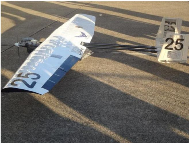
**Figure 3.3.1: UFPR aircraft implementing two carbon fiber tubes connecting the aft to the**
