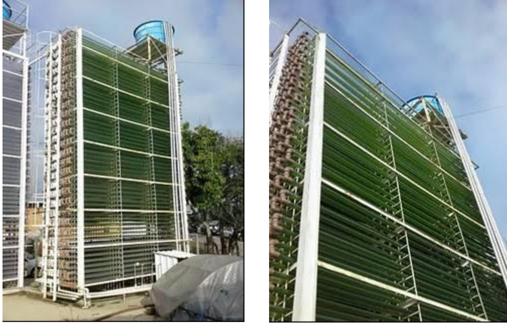
Figure 4 - Appearance of the first industrial scale photobioreactor of NPDEAS at UFPR (5 m x 2 m x 8 m).
