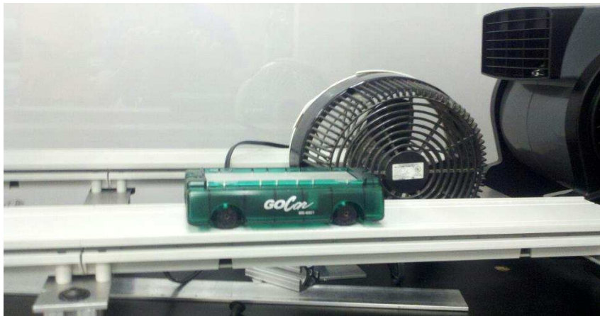
Figure 2 - Cart used in Wind Tunnel
