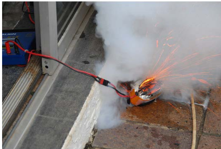
Figure 12.1: LiPo Battery Explosion
