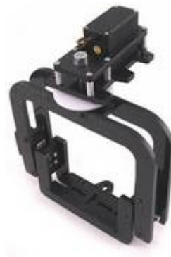
Figure 9.15: Pan / Tilt Camera Gimbal Design Concept
