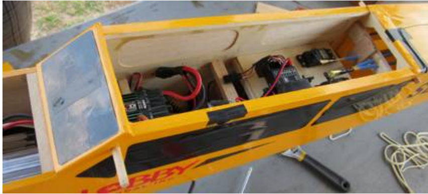
Figure 9.2: Components installed in Telemaster
