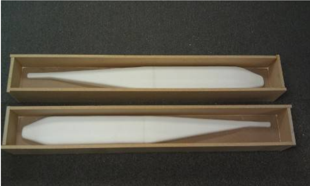
Figure 6.2: Boxes for construction of fuselage mold
