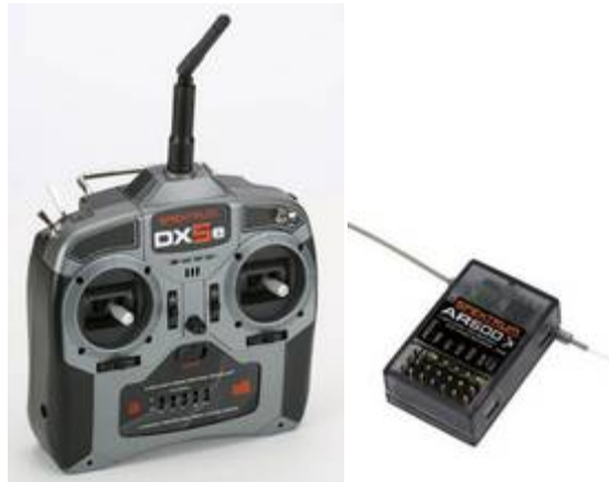
Figure 5.27: Spektrum RC transmitter (left) and receiver (right)
