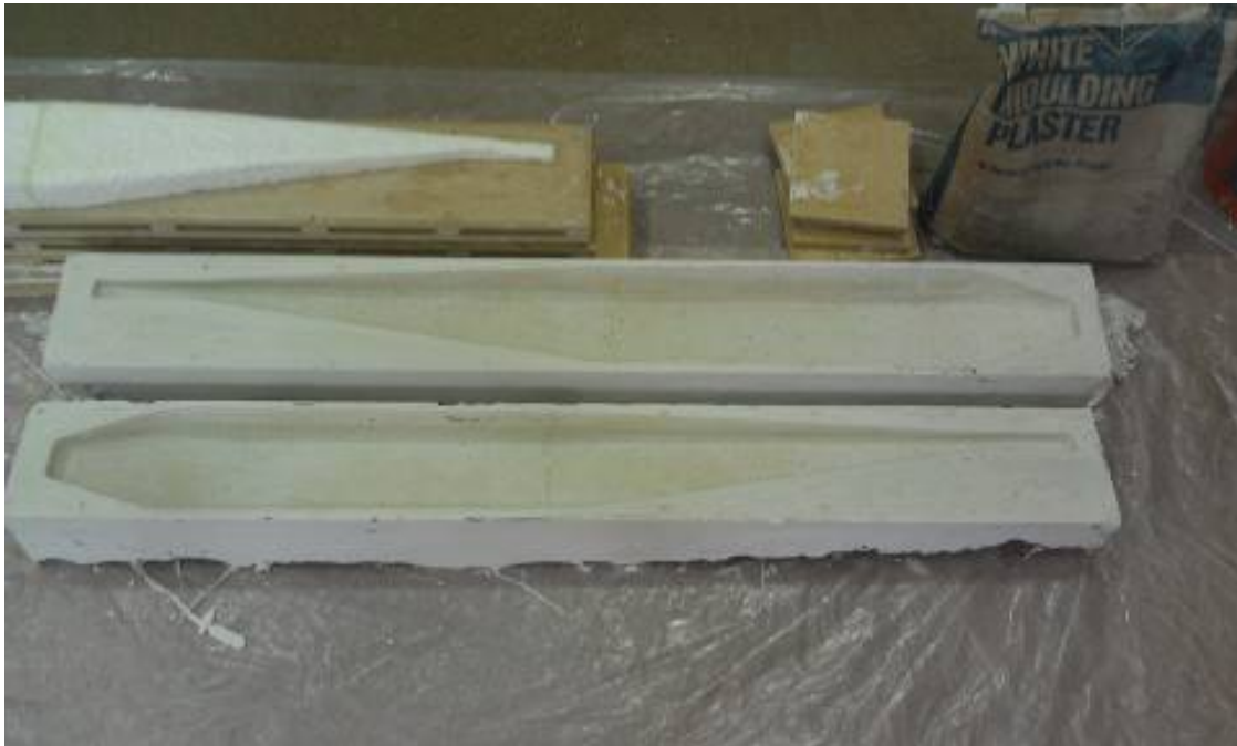
Figure 6.3: Plaster mold after removal from box
