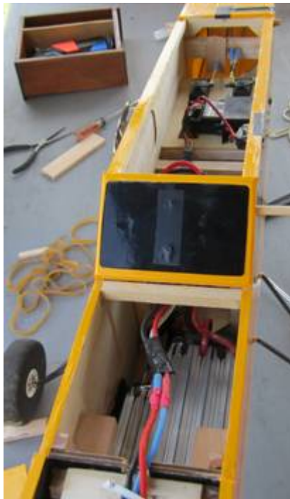
Figure 9.3: Batteries installed in Telemaster
