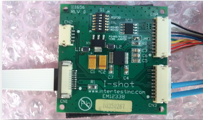
Figure 6.12: I-shot Block camera Interface board
