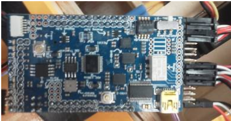
Figure 6.4: Autopilot Board connected to servos
