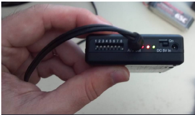
Figure 6.9: Bottom of Video Rec. With correct pin settings
