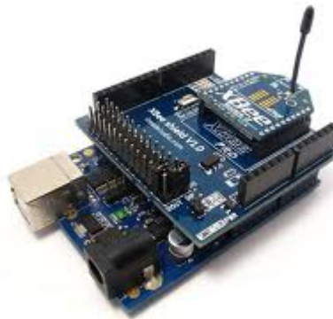
Figure 13 Arduino UNO with mounted XBee radio kit
