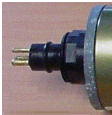
Figure3.5.1.1: RMG-3FS Connector on SBE-4
