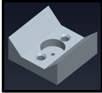
FIGURE 28: THE V-BLOCK (CUP) THAT WILL BE USED IN THE KINEMATIC COUPLING DESIGN
