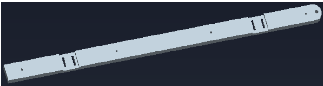
FIGURE 25: SHOWS THE ALUMINUM 6061 BRACKET THAT WILL BE APPLIED ALONG THE EDGES OF THE BOTTOM OF THE PANELS
