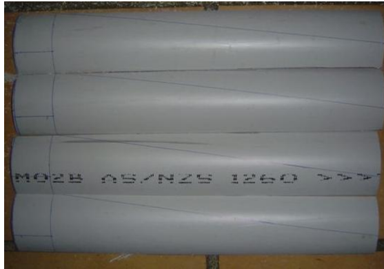
Figure 94 – Sample PVC cuts to approximate airfoil shape. "YourGreenDream - Homemade Solar, Wind and Green Power Diy Projects to Generate Energy. How to Make PVC Windmill Blades." YourGreenDream - Homemade Solar, Wind and Green Power Diy Projects to Generate Energy. Web. 07 Dec. 2011. < http://www.yourgreendream.com/diy_pvc_blades.php >.
