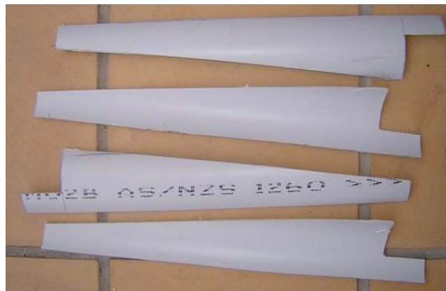
Figure 10 – Sample PVC cuts to approximate airfoil shape. "YourGreenDream - Homemade Solar, Wind and Green Power Diy Projects to Generate Energy. How to Make PVC Windmill Blades." YourGreenDream - Homemade Solar, Wind and Green Power Diy Projects to Generate Energy. Web. 07 Dec. 2011. < http://www.yourgreendream.com/diy_pvc_blades.php >.
