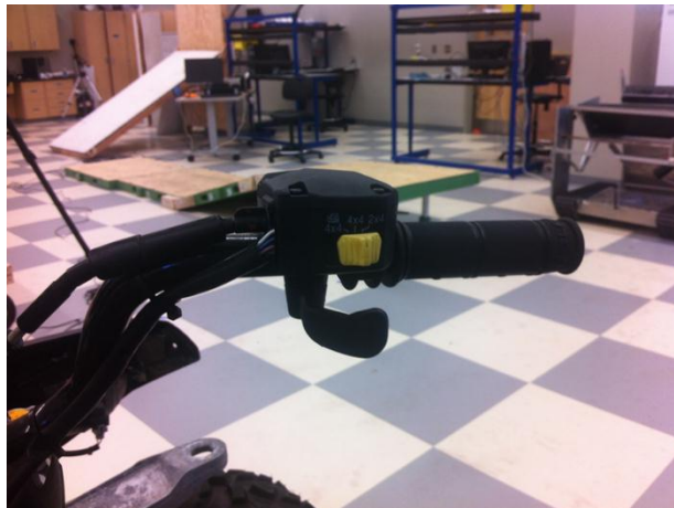
Figure 15 – Factory installed throttle actuator mechanism
