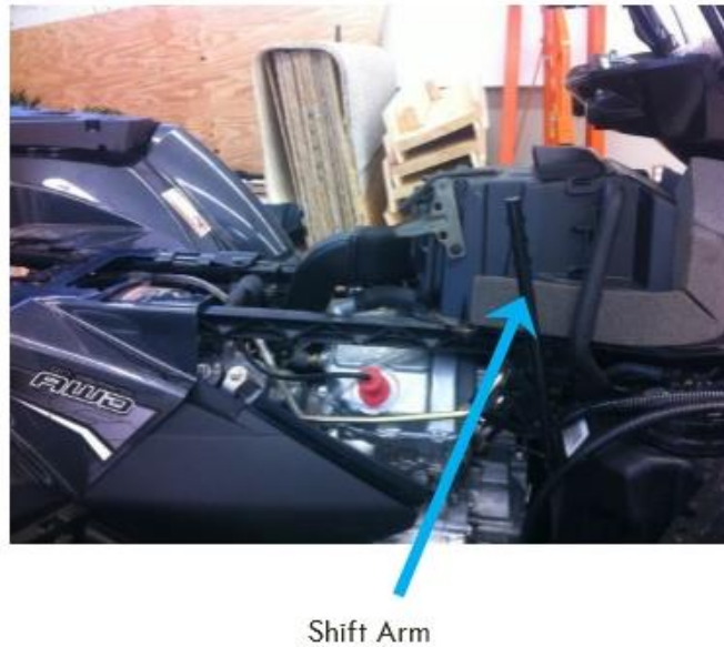
Figure 4 – Gear Select Mechanism with arrow point to shift arm
