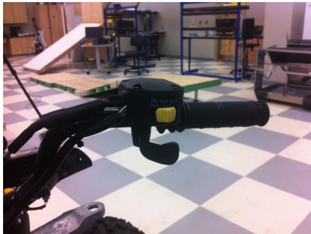
Figure 19 – Factory installed throttle actuator mechanism
