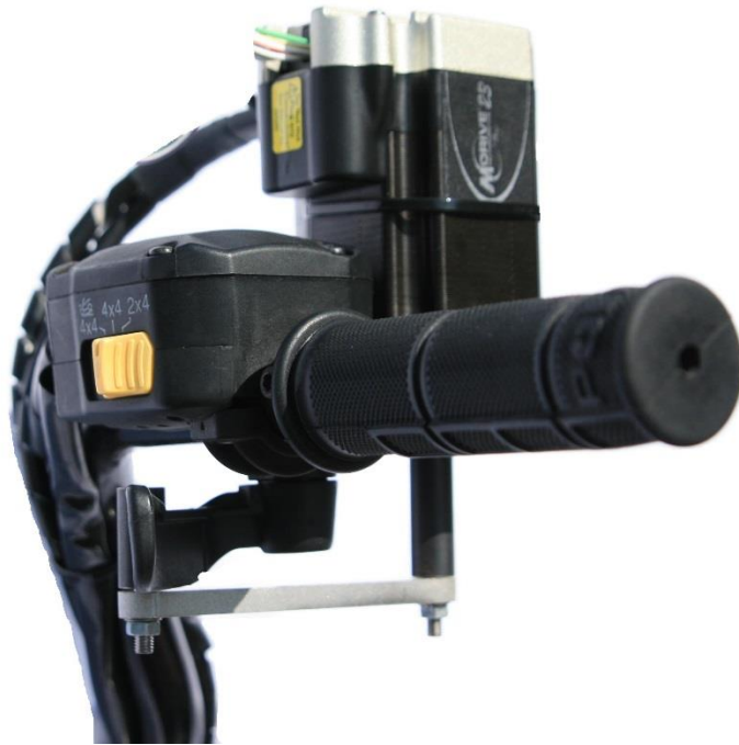
Figure 23 – Fully assembled Gear Select manipulation design
