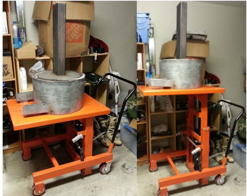
Figure – The cart at its fully-lowered (left) and fully-raised (right) positions with the main canister housing set on top.
