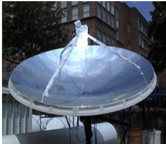
Figure 7: Solar concentrating dish used to generate steam
