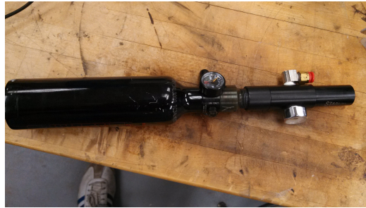
Figure 16: Air tank with regulator
