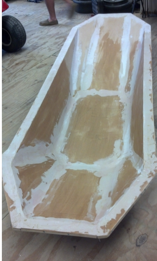
Figure 3.4: Completed MDF Top Chassis Mold
