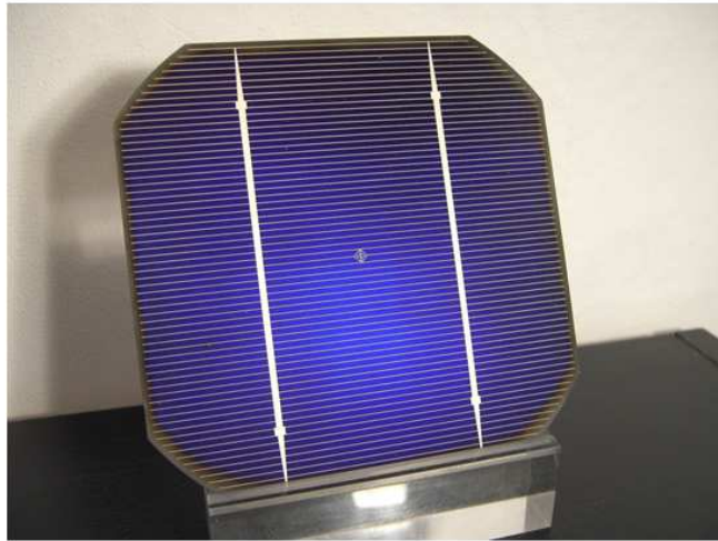
Figure 3.20: 125x125mm Mono-Crystalline Solar Cell
