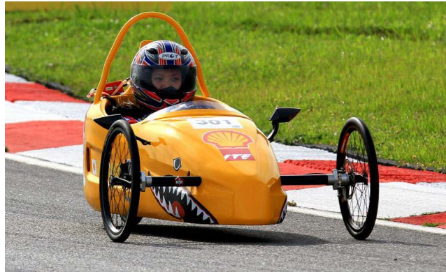
Figure 3.10: Rigid Suspension Example
