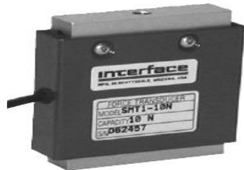
Figure 28- Interface Load Cell-SMT1-10N
