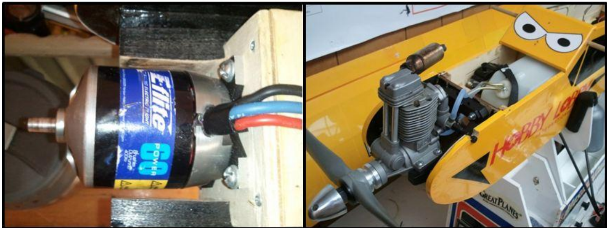
Figure 1 Left: DC motor that used to be on plane. Right: Magnum XL mounted on plane and fuel tank installed.
