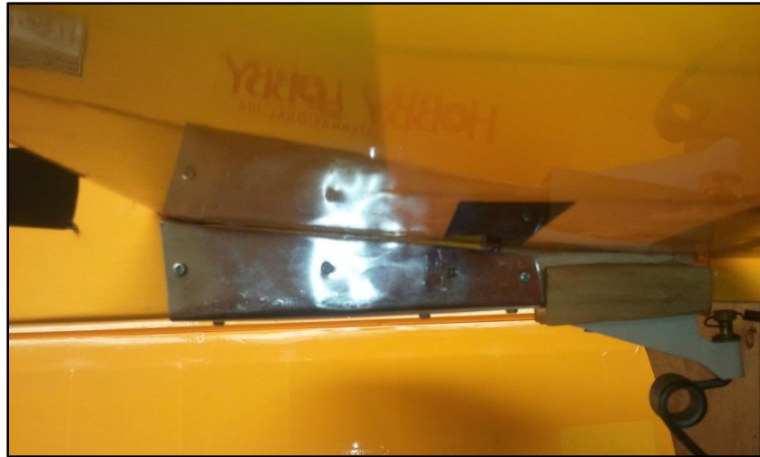
Figure 8: Tin bracket reinforcing the tail portion of the fuselage
