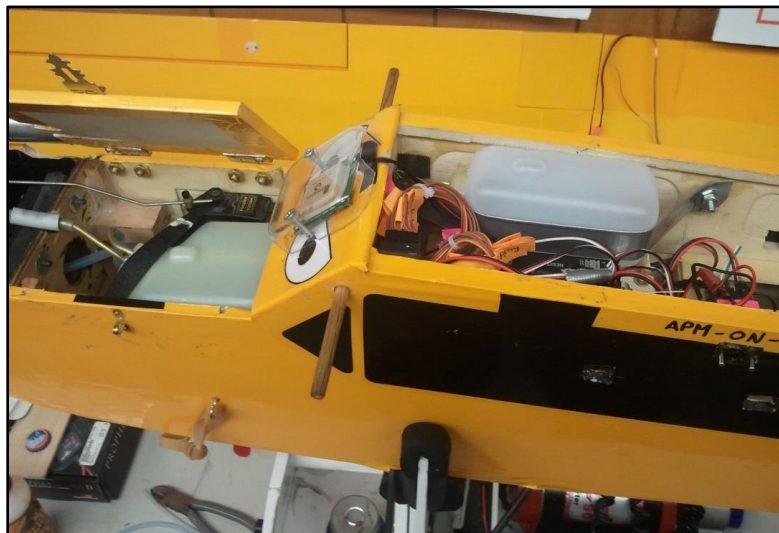
Figure 5: Dual fuel tanks: main tank (left), feeder tank (right)
