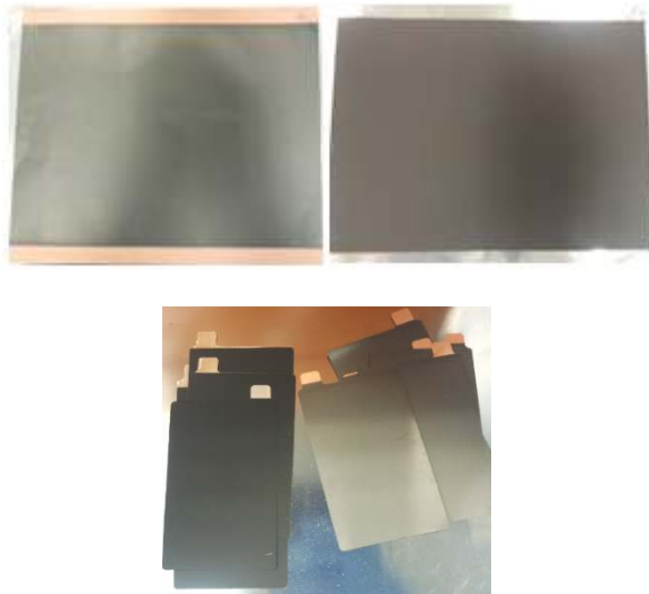
FIGURE 18. ELECTRODES BEFORE AND AFTER CUTTING
