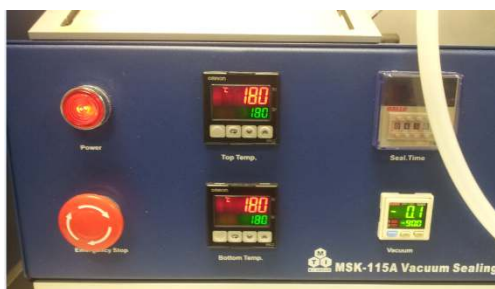
FIGURE 28. CONTROLS OF VACUUM SEALER
