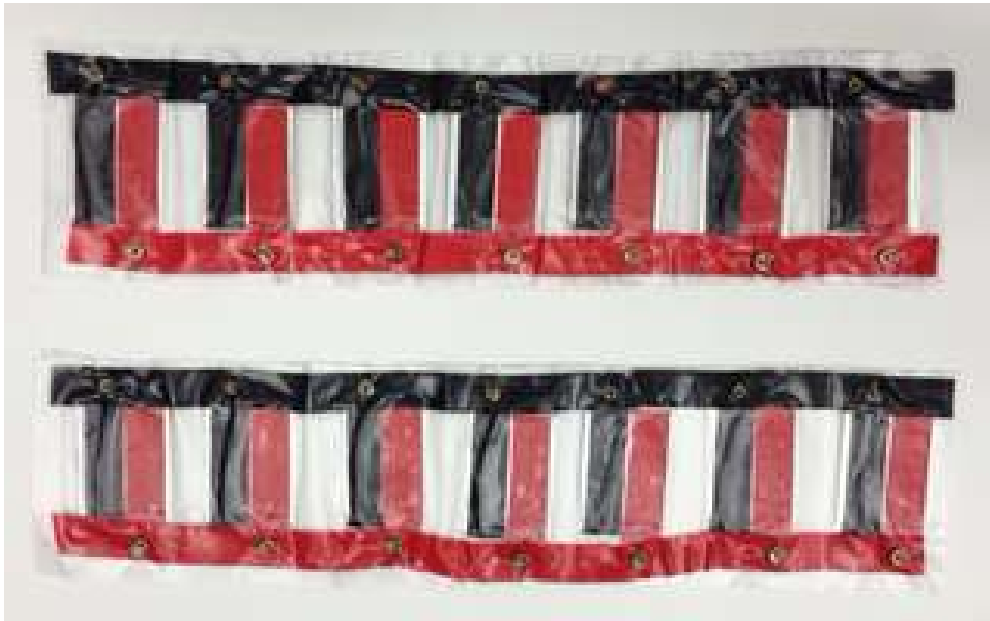
FIGURE 14: RAW CELLS CONNECTED IN PARALLEL
