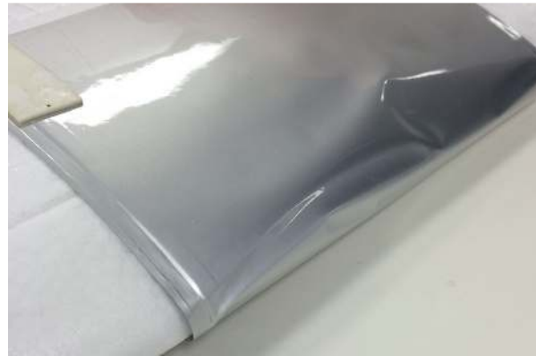
FIGURE 12: BATTERY BENT AROUND AIRFOIL
