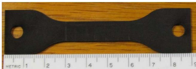
Figure 8: Black Rubber in Dumbbell Geometry
