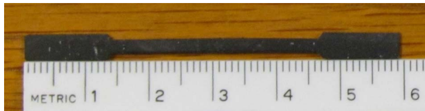
Figure 9: Dogbone Geometry of C5270
