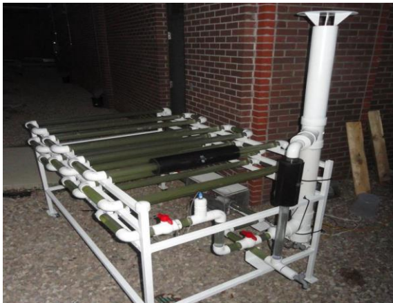
Figure 2 shows the Photobioreactor created last year. It incorporated sensors to monitor the microalgae growth. (Senior Design Project)
