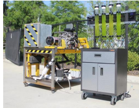
Figure 1 shows the Trigenator System with Photobioreactor. This was completed by the 2011 Senior Design team. (Senior Design Project)
