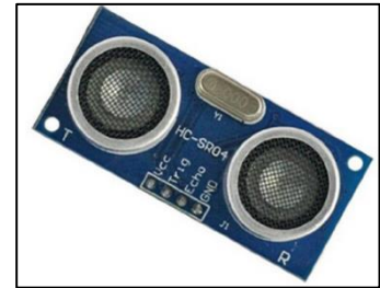
Figure 5 shows the ultrasonic sensor used in the improvement of our mass flow sensor.
