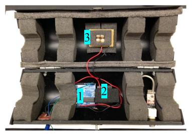
Figure 12 Concentration Sensor Hardware: 1. Arduino Microcontroller; 2. Wheatstone Bridge (LDR1, LDR2, R1, R3) & Control LED (LED5, R2); 3. Test LED's (LED1-4, R4-7)
