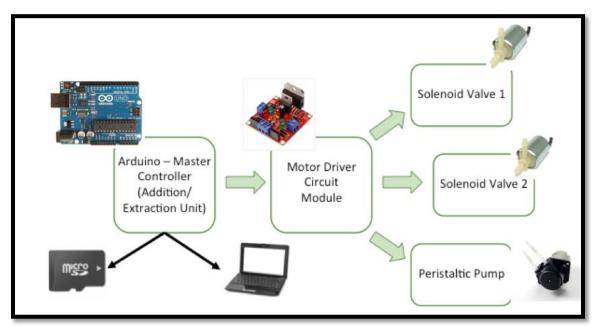
Figure 13 Addition/Extraction Component Schematic
