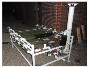
Figure 2 shows the Photobioreactor created last year. It incorporated sensors to monitor the microalgae growth. (Senior Design Project)
