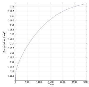
Figure 8 – A extended graph of the normal operating conditions. The system does not experience a duty cycle longer than 600 seconds. This simulation was done to determine the initial temperature during the transient case.
