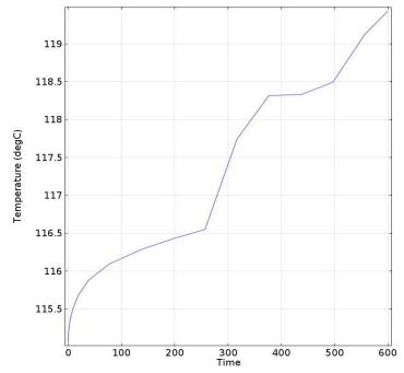
Figure 9 – The transient model. The first 300 seconds was 1W of heat generation and then from 300 – 600 seconds the overdrive occurred. The phase change can be seen to occur at 375 – 500 seconds.
