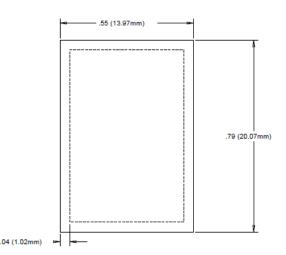
Figure 3. Heatsink geometry selected for prototyping.
