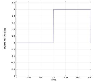
Figure 7 – The duty cycle that the COMSOL model experiences in the simulation. The normal operation parameter is 1W and the overdrive is 2W.
