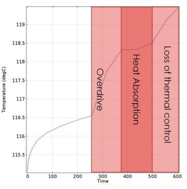
Figure 4. Temperature (in °C) as a function of time (in seconds) of the PCM as calculated by COMSOL.
