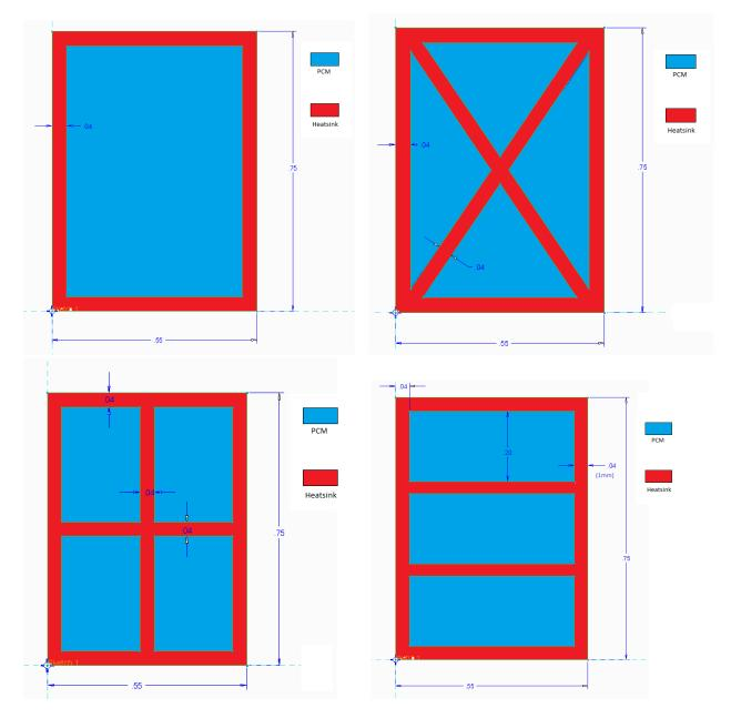
Figure 5. The four proposed designs for the heatsink housing. Analysis in COMSOL found that the design in the upper-left was optimal.
