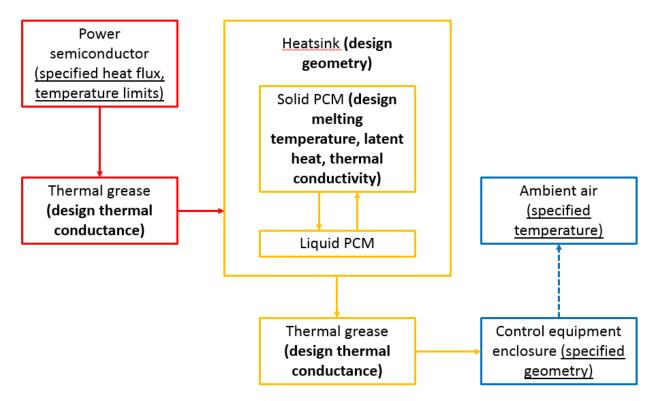
Figure 1. General schematic of heat transfer within control equipment assembly. Underlined words indicate sponsorspecified parameters, bold words indicate free design parameters. Arrows indicate desired direction of heat transfer. Solid arrows indicate conduction, dashed arrows indicate natural convection.
