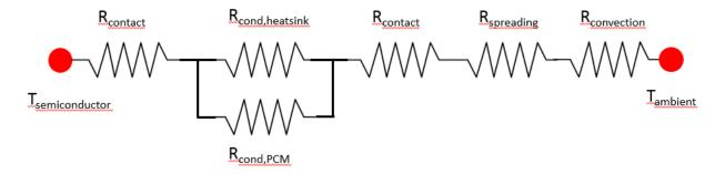
Figure 2. Schematic of thermal resistance network for steady-state analysis.
